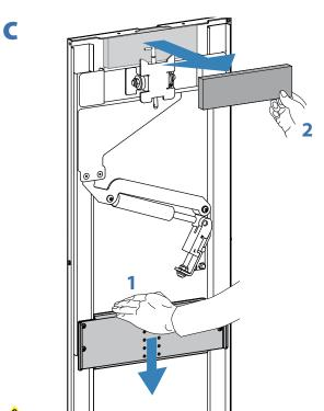
WARNING: Injury may result if the cardboard spacer is removed without first lowering the keyboard bracket. DO NOT remove the cardboard spacer before lowering the keyboard bracket.
